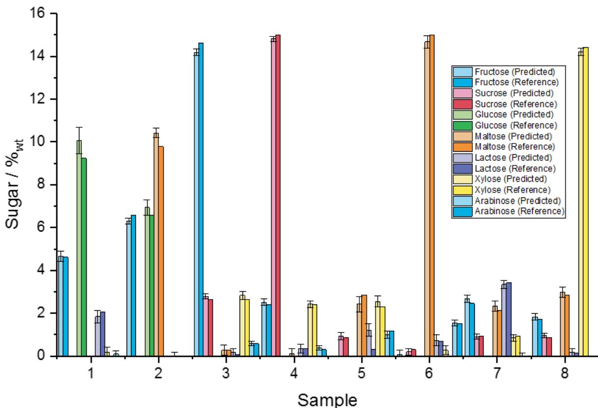
**Figure 3:** Predictions for mixtures of sugars using the IRmadillo and a pre-built PLS model.
