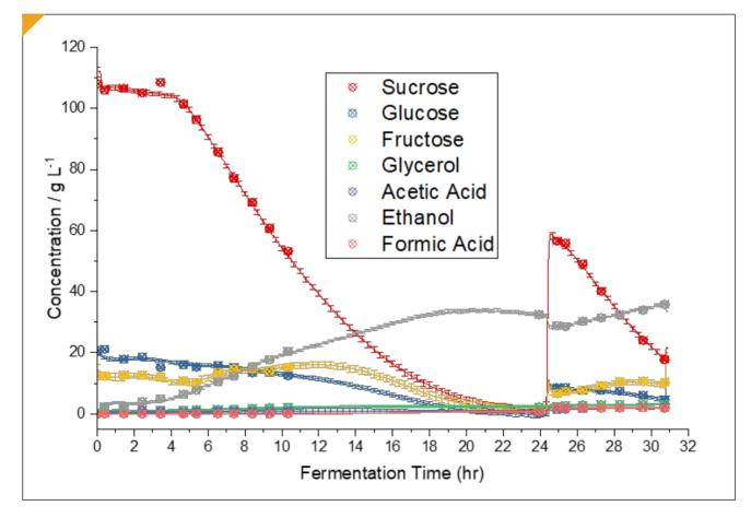
**Figure 1:** Plot of chemicals monitored by the IRmadillo during a fermentation process over 32 hrs clearly showing ability of the instrument to monitor multiple species simultaneously (sugars, acids, and alcohols).
