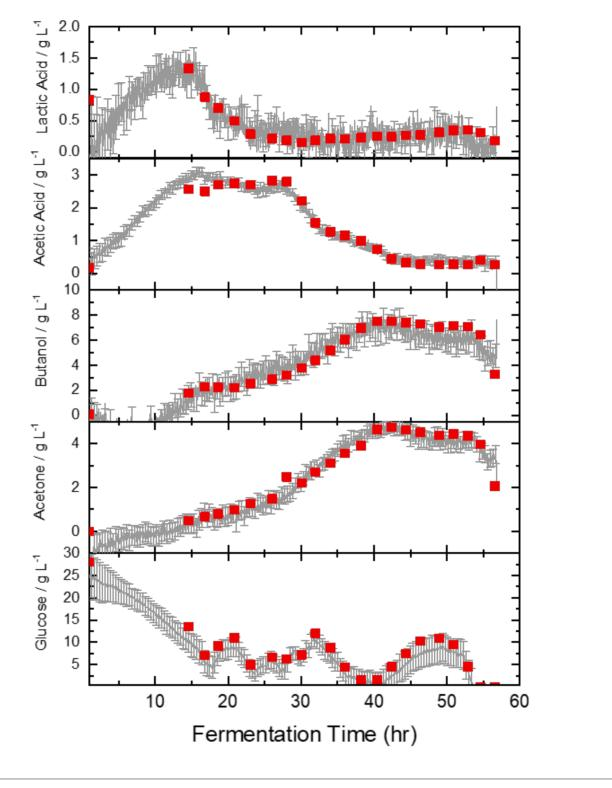
**Figure 2:** Prediction of reaction constituents throughout an ABE fermentation process with reference values from HPLC. The IRmadillo can be used for in-process PAT to effectively monitor a range of biochemical reactions for industrial applications.
