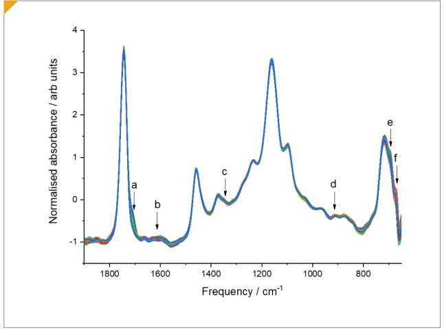
Figure 1: Spectra acquired on the IRmadillo during calibration of FFA and FAME mixtures in sunflower oil.
