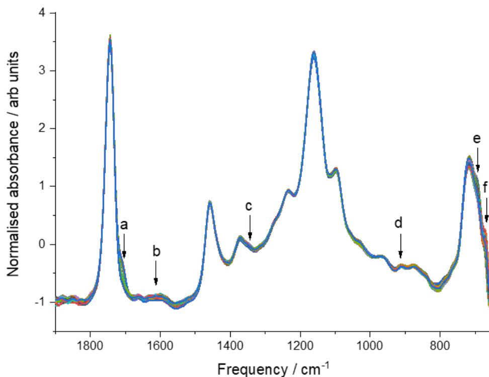
**Figure 1:** Example spectra of a mixture of triglyceride feedstocks. Band assignment: a) C=O in FFAs, b) C=C bonds in unsaturated FFAs and FAMES, c) C-H bends in FFAs and FAMES, d) C-C and C-O stretches in FFAs and FAMES, e) O-C=O bend in FFAs, f) O-C=O bends in FFAs and FAMES
